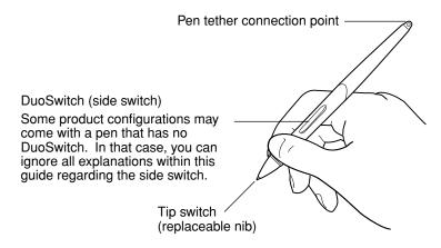
**Note:** When the pen is not in use, place it in the pen tray, the pen storage compartment, or lay it flat on your desk. To maintain the sensitivity of your pen, do not store the pen in a container where it will rest on its tip.
